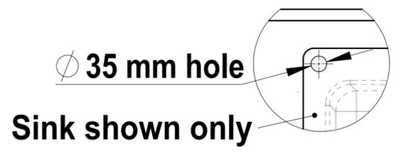
Position the Tap such that it dispenses into the sink bowl with ample clearance for a cup or a carafe. Alternatively, the Tap could be mounted away from the sink using a Font, available as an accessory.
